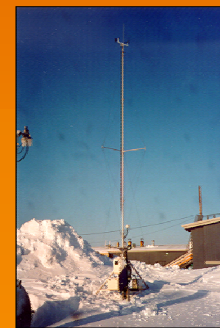
[Fig.5] NEWNET (Neighborhood Environmental Watch NETWORK), uses these towers to gather radiation and meteorological data. This tower is located in Barrow.
